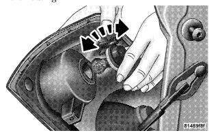
**Rotating Bulb Socket From Housing**
